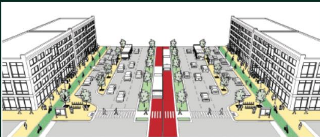
TYPICAL CROSS SECTION: 14 MILE TO QUARTON RIGHT-OF-WAY = 200'
