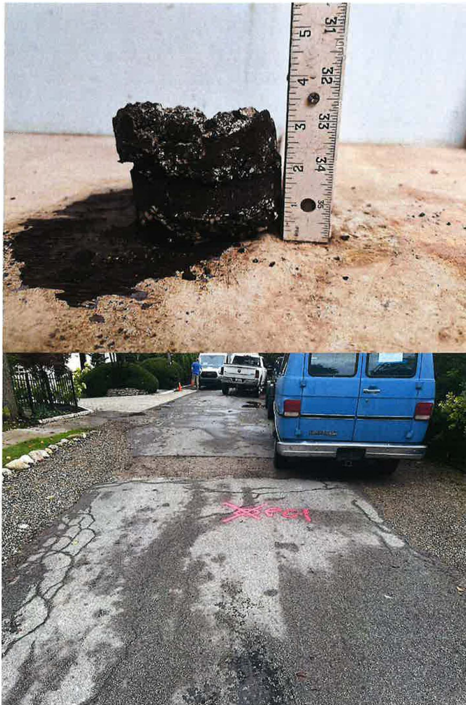
Core Photograph of PC-1: Bituminous Concrete = 3 inches
