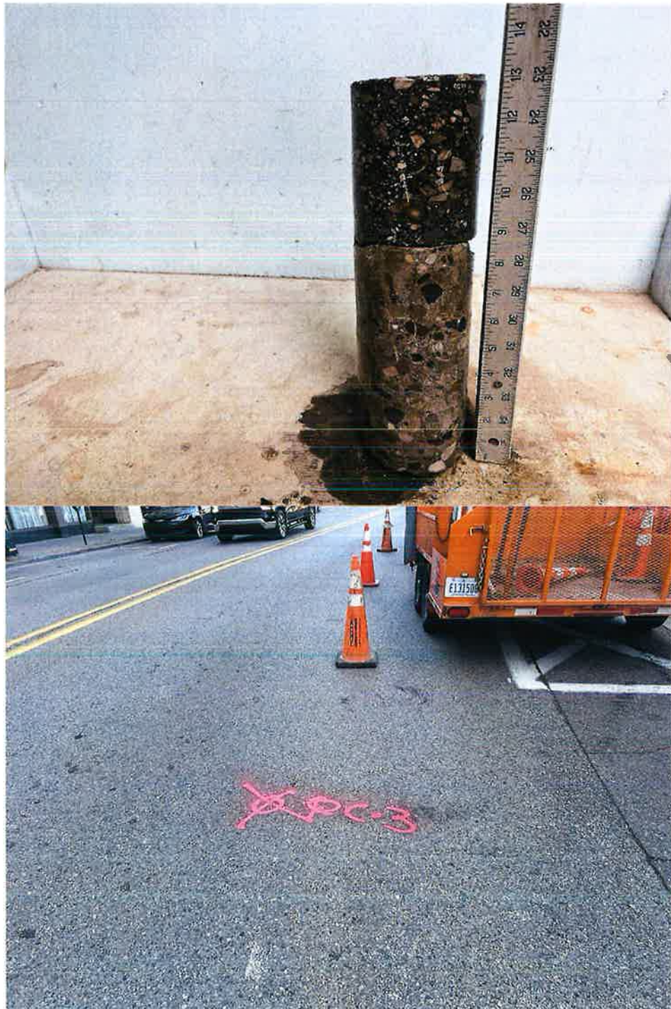
Core Photograph of PC-3: HMA Pavement = 4-1/2 inches PCC Pavement = 8-1/2 inches
