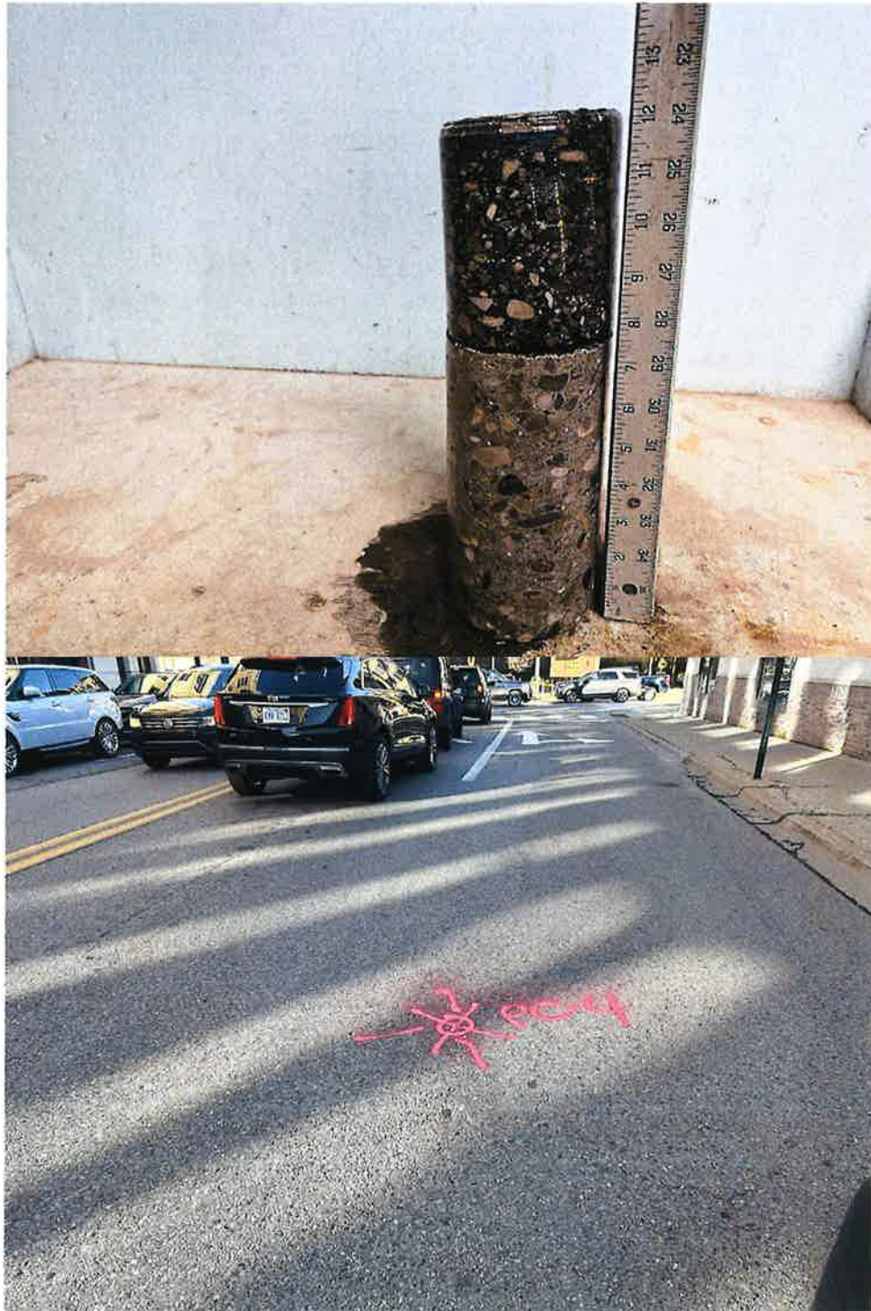
Core Photograph of PC-4: HMA Pavement = 4-1/2 inches PCC Pavement = 7-1/2 inches
