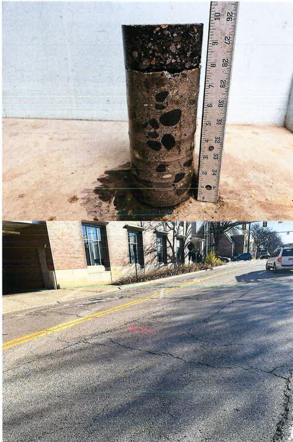
Core Photograph of PC-1: HMA Pavement = 2 inches PCC Pavement = 7-3/4 inches
