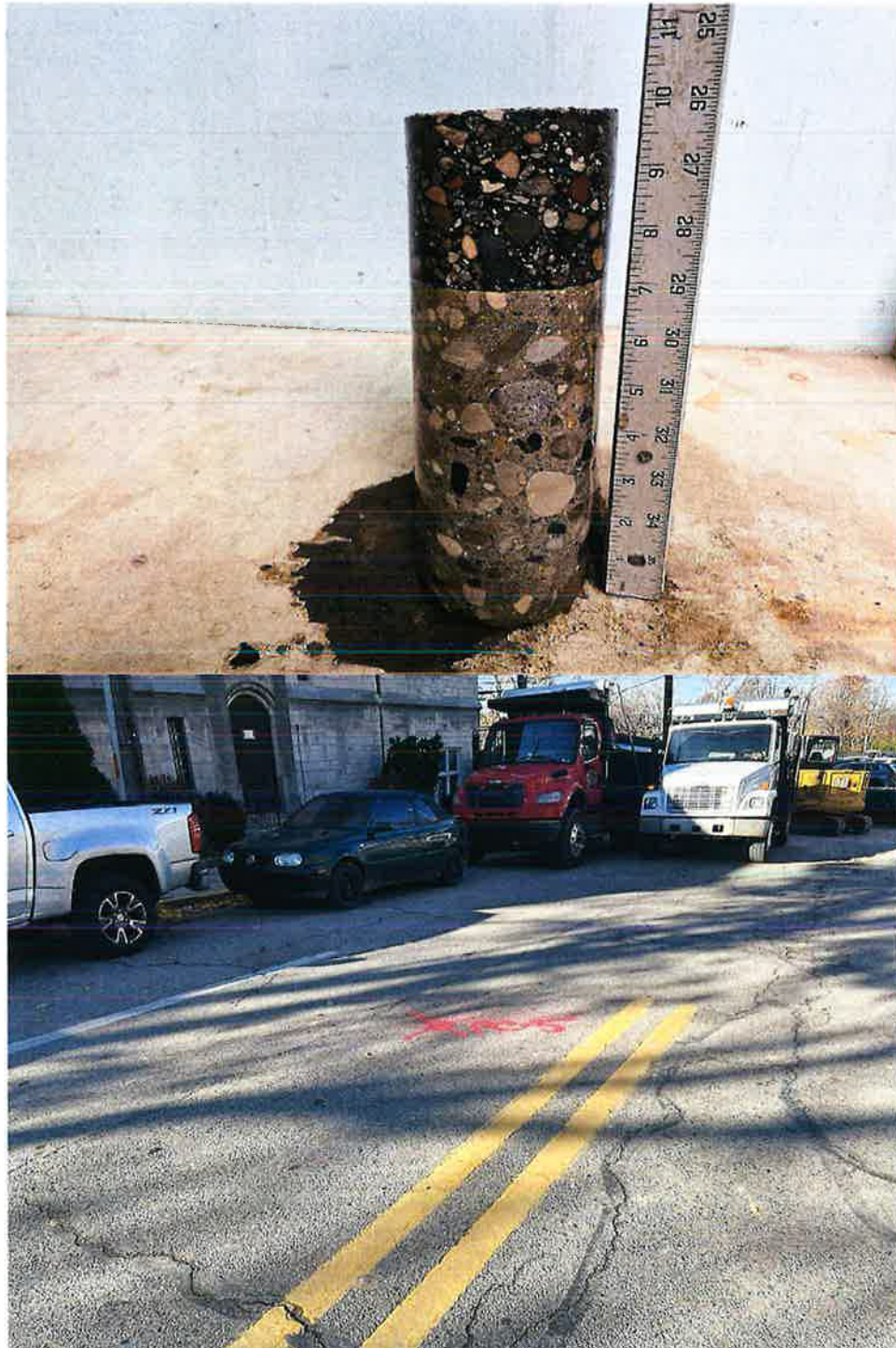
Core Photograph of PC-5: HMA Pavement = 3 inches PCC Pavement = 7 inches
