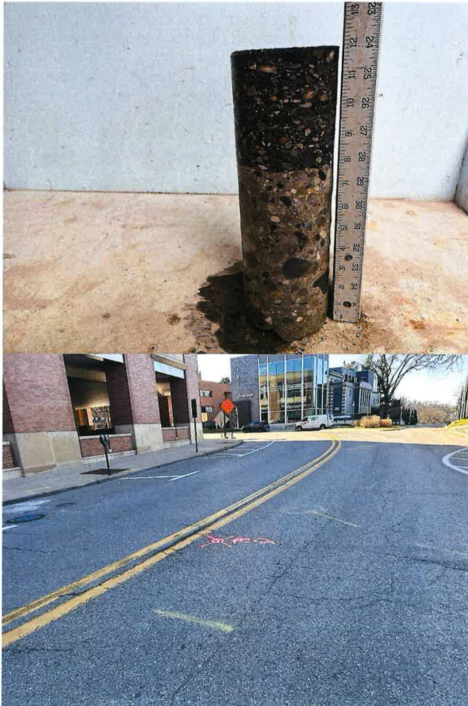
Core Photograph of PC-2: HMA Pavement = 4-1/2 inches PCC Pavement = 7-1/2 inches
