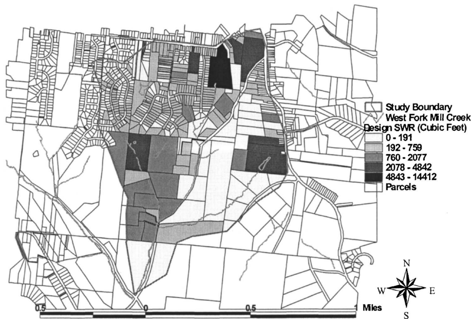
Fig. 2. Excess stormwater runoff
