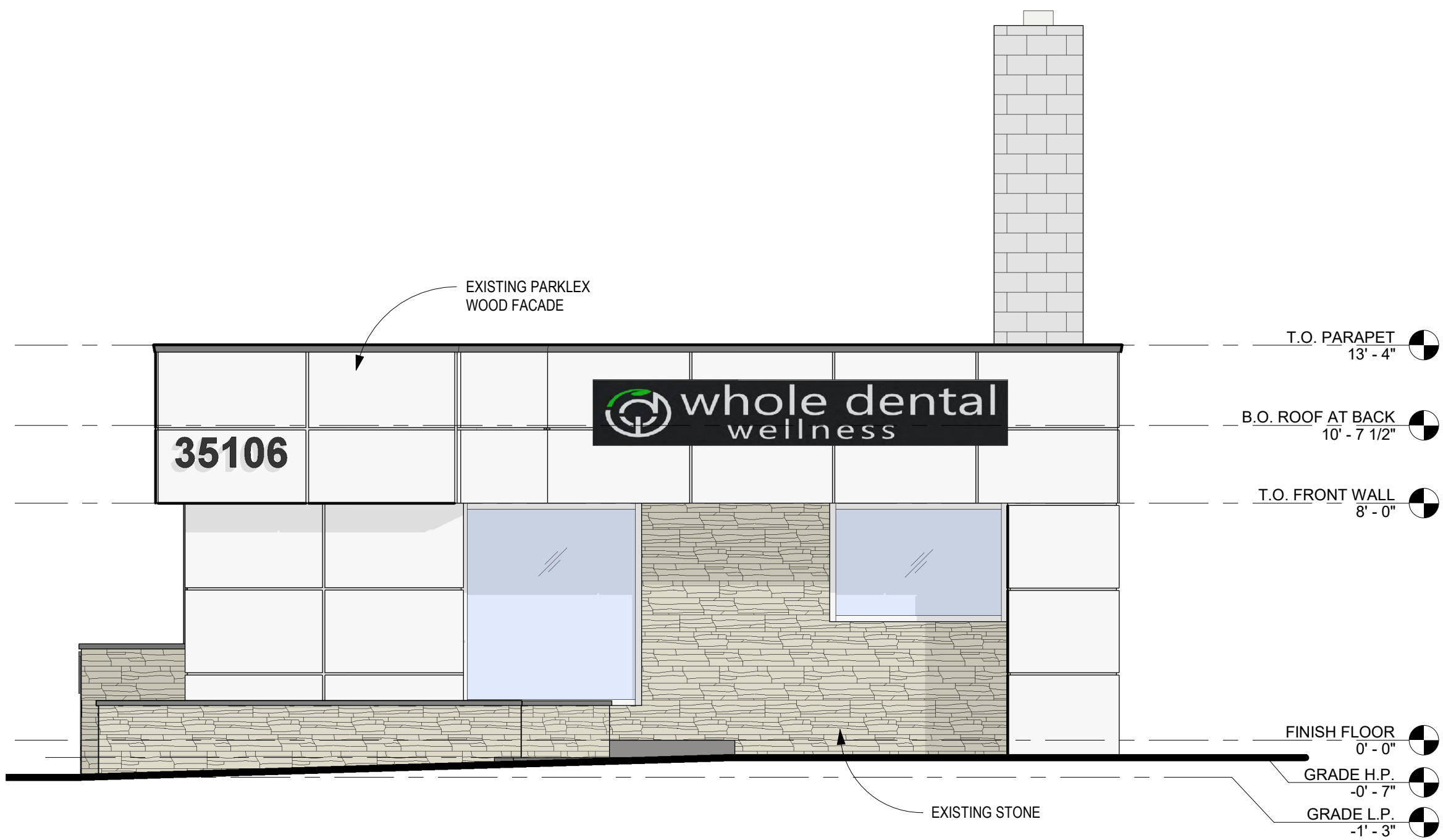
EXISTING FRONT ELEVATION 1/4" = 1'-0"
