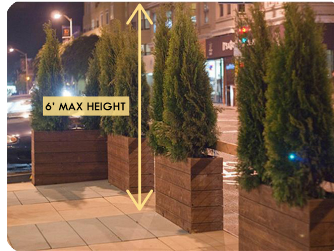
Figure 5. Max planter and plant height is 6 feet.
