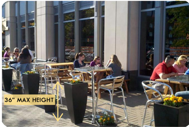
Figure 4. Max height of barriers is 36 inches.
