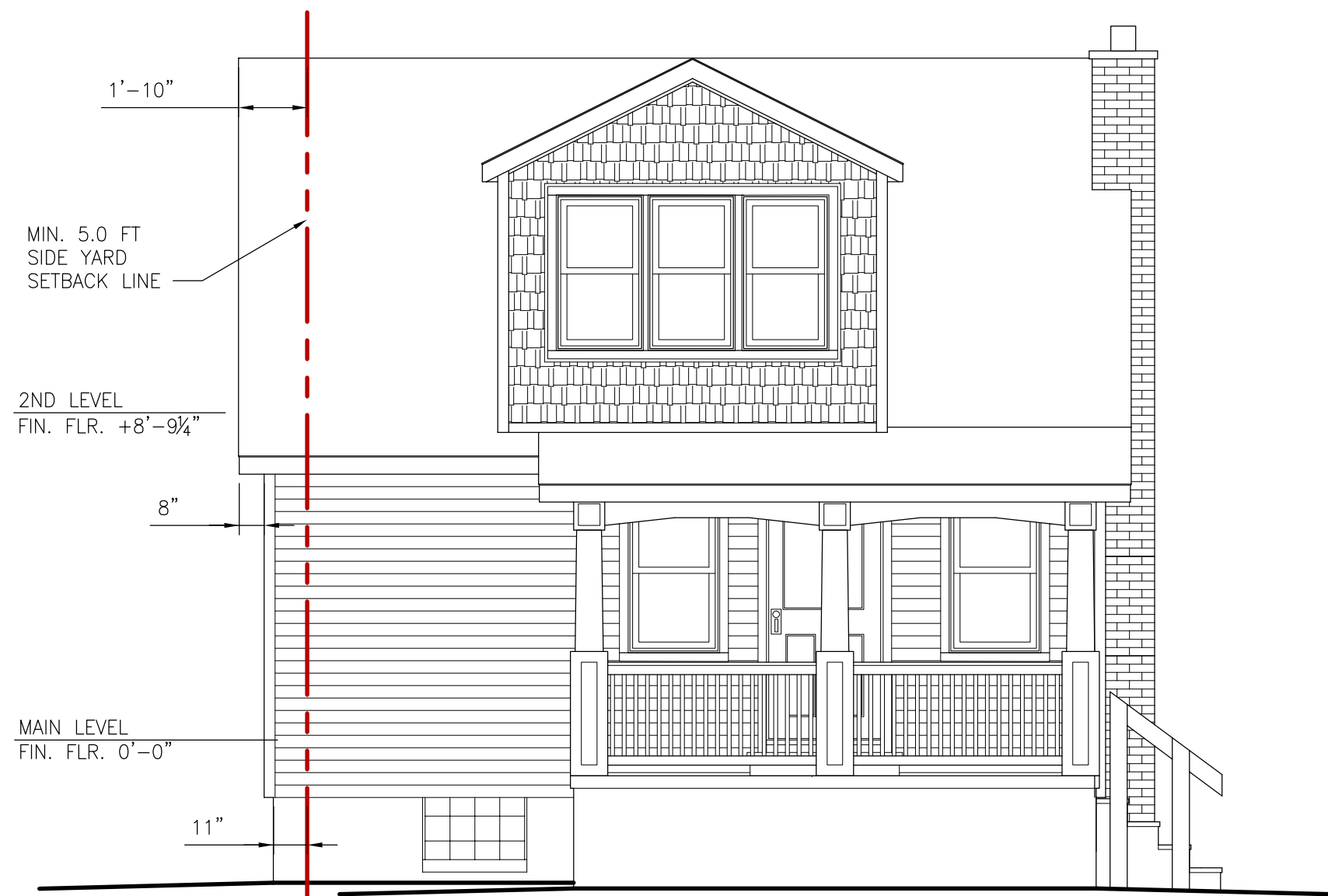
SOUTH (FRONT) ELEVATION SCALE: 1/4" = 1'-0"
