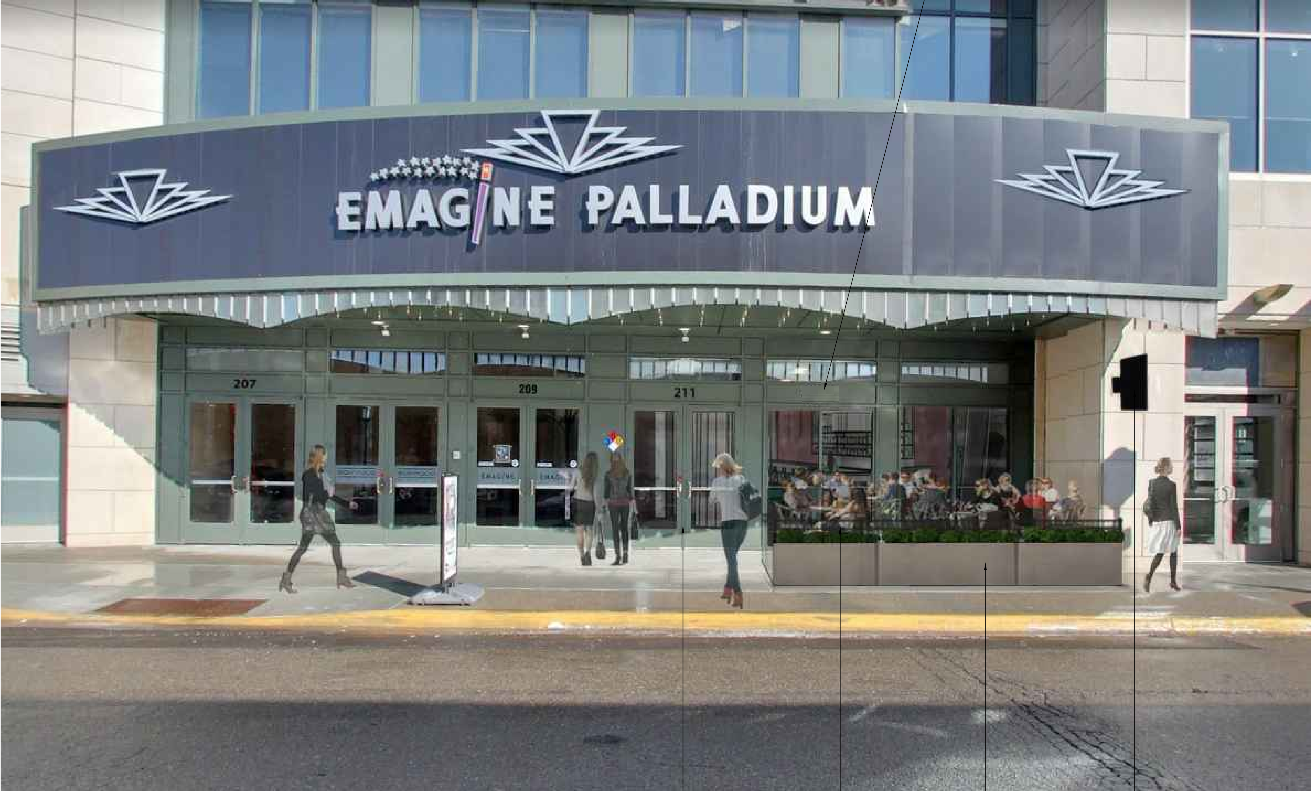
42" HIGH ALUMINUM FENCE EXISTING GLASS AND ENTRY DOORS TO REMAIN PROPOSED 30" ALUMINUM POWDER COATED PLANTER BOX EXISTING SIGN TO BE UPDATED -SEE SIGN DETAIL "B"
