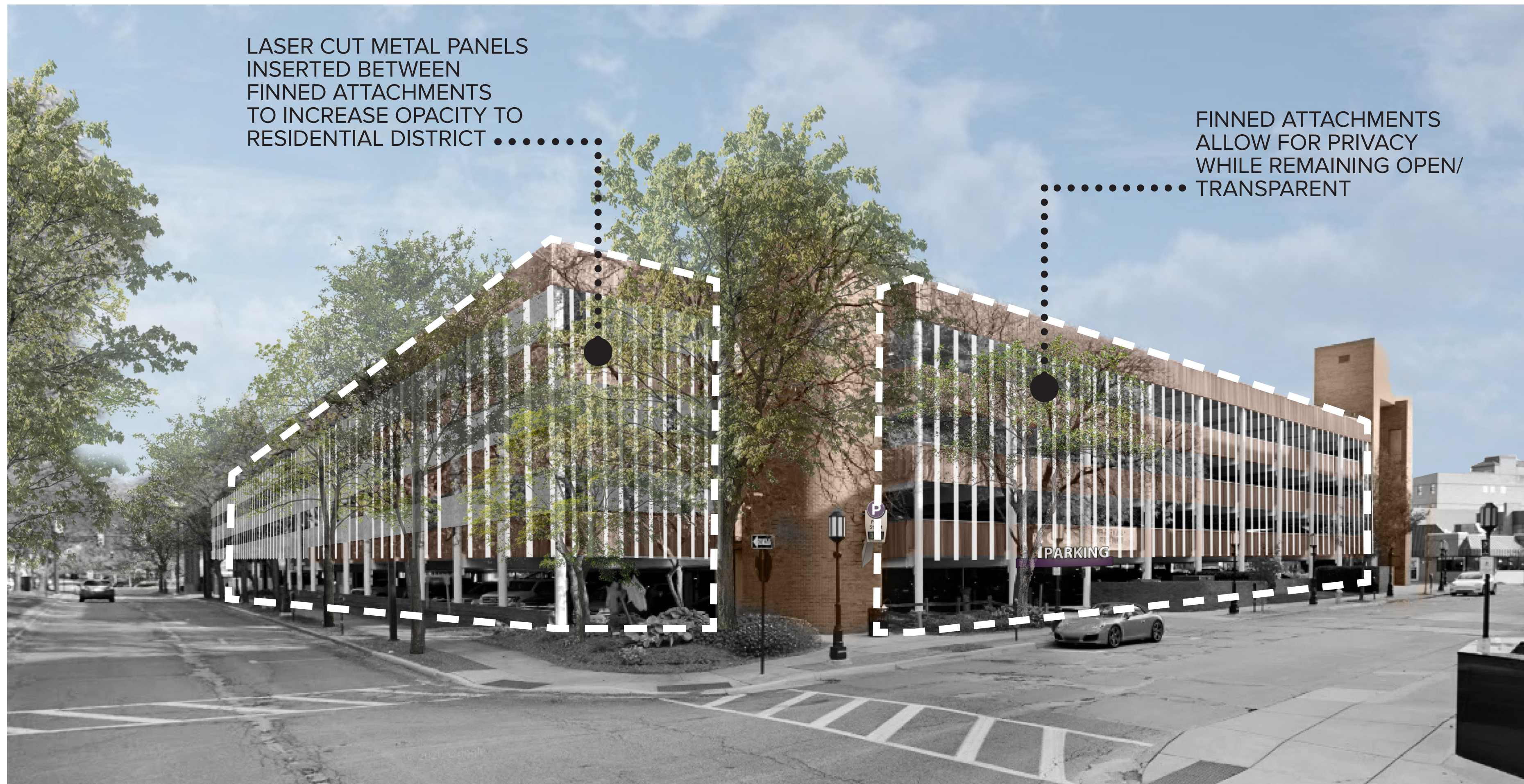
FACADE 1 - VERTICAL FINNED FACADE W/ LASER CUT METAL PANELS
